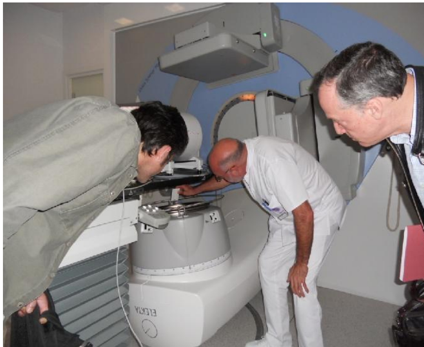
Professor Ion Christian Chiricuta explaining the multileaf collimator of the linear accelerator at the Amethyst Center
