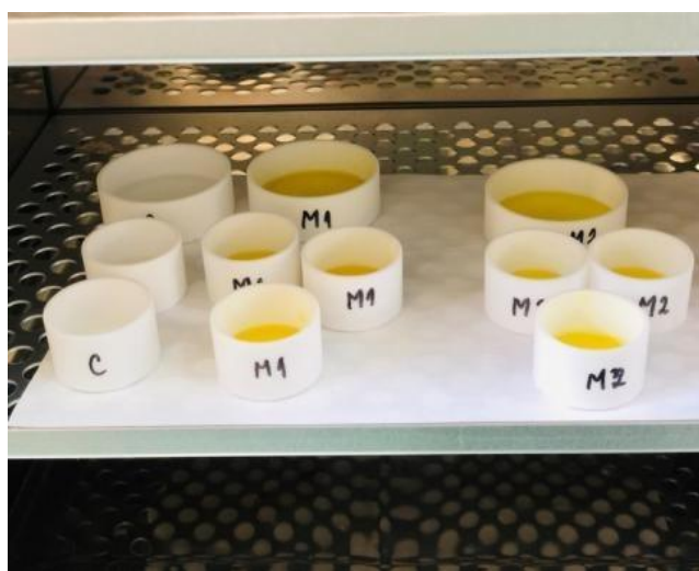
Figure 9.2. Step in membrane manufacture; Addition of cross-linking agent and deposition in Teflon Petri dishes for drying.
