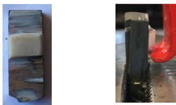
Fig. 4.5 – The alloy samples on which the ceramic mass was applied, prepared for testing the metal-ceramic bond
