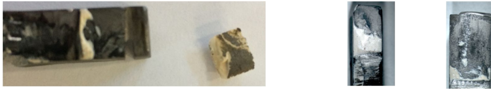
Fig. 4.6 – Appearance of the tested samples after failure of the metal-ceramic bond.
