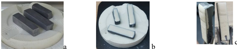
Fig. 4.4 – The appearance of the experimental alloy rods: a) at the end of the oxidation program, b) after applying of the opaque layer, c) after applying of the first ceramic layers
