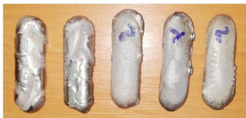
Fig. 6.2 – MoNbTaTiZr ingots, high entropy alloy, obtained using the "RAF MRF ABJ 900" facility
