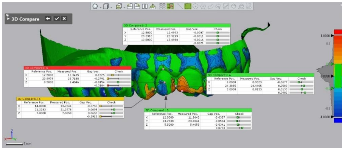
Figure 7.4 – Example of measurements made in the comparison between the digital wax-up and the initial clinical situation.
