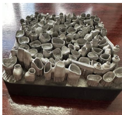
Figure 6.1. Post attachment pins on the 3D metal printer platform (personal archive)
