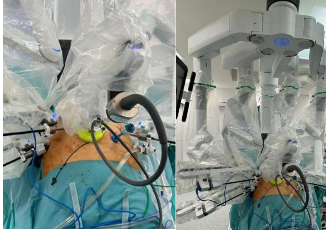
Figure 10.4 Positioning of the robotic arms
