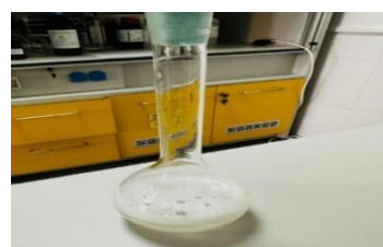
Figure 4.13. Precipitation of the filtrate combined with 0.9 M NaCl
